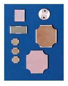
AMC X2Y® capacitor products employ a unique, patented internal design in which common shielding electrodes form a Faraday Cage around traditional capacitor electrodes. This nearly eliminates parasitics and creates two matched capacitors that are immune to temperature, voltage and aging performance differences. Available X2Y® products include planar capacitor arrays, discoidal capacitors, and large format chip capacitors offering the following performance advantages:
